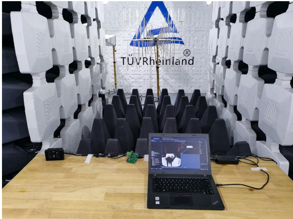
Photograph 6: Set-up for Radio-Frequency Electromagnetic Field (RS)
