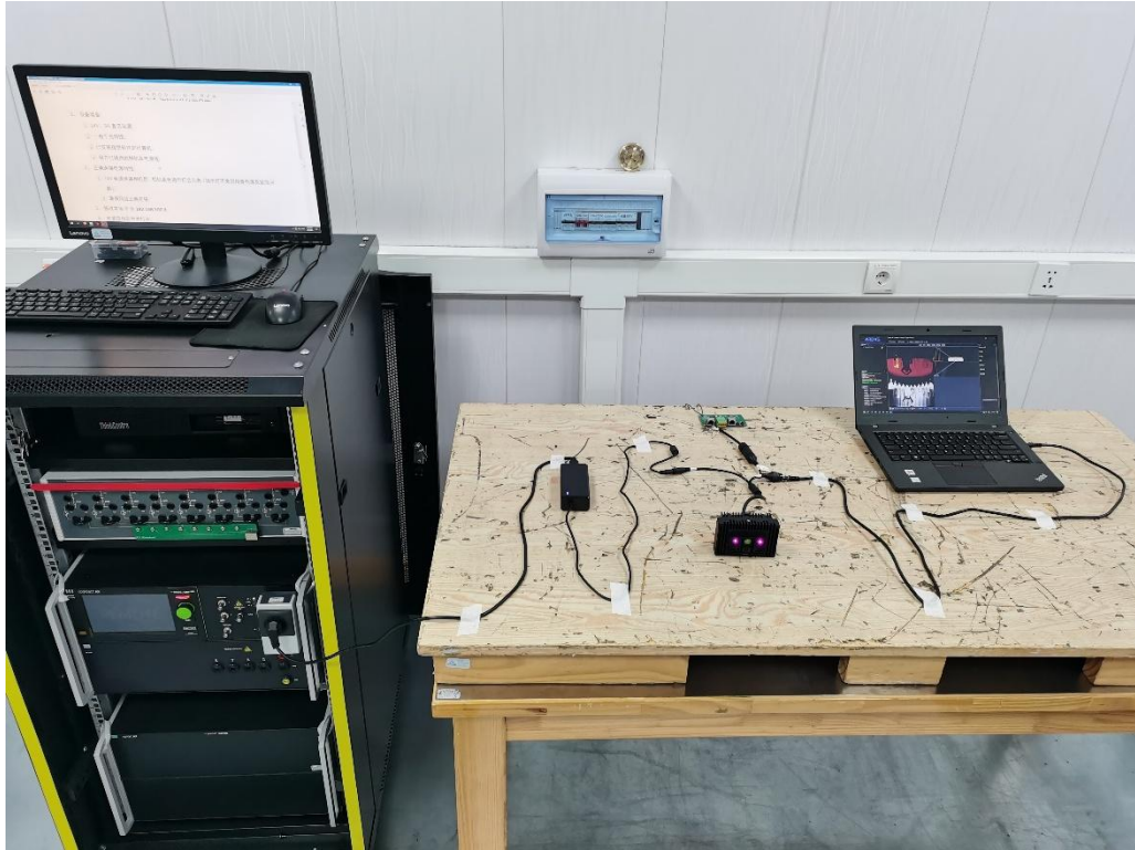
Photograph 7: Set-up for EFT AC mains
