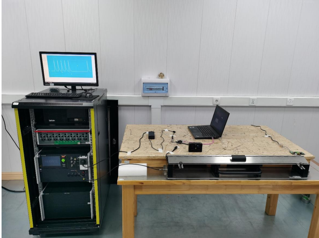
Photograph 8: Set-up for Surge AC mains
