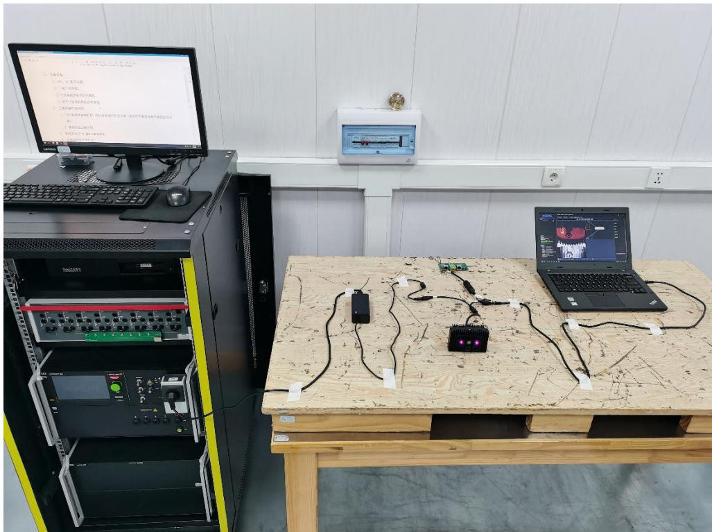
Photograph 8: Set-up for Surge AC mains
